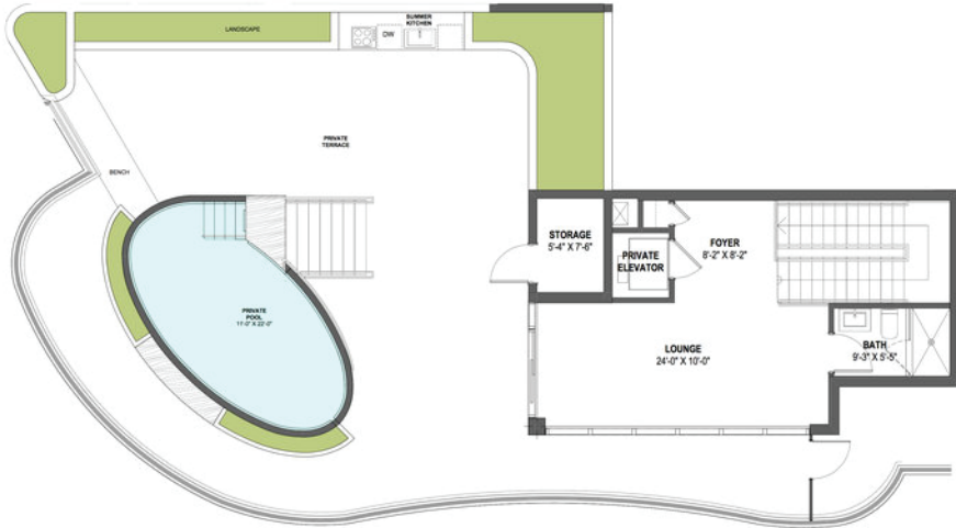
UNIT UPH-01 pool deck level level 64 - floor plan 1/4" = 1'-0"
